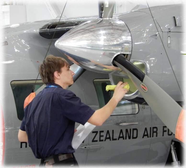
Michael is undertaking the engine intake and propeller inspection of a Mitsubishi MU2 as part of the daily inspection module at the selection competition .
