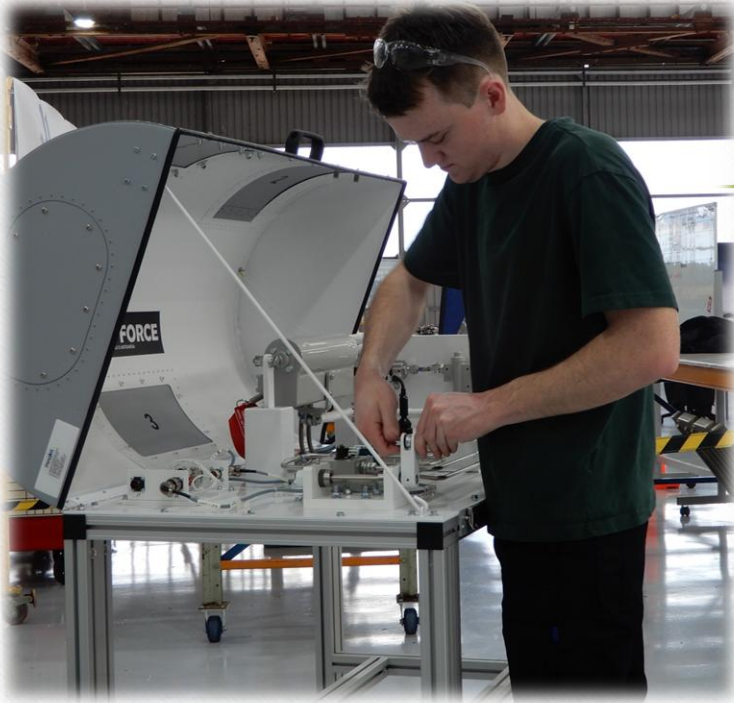
Tim is refitting a flight control rod to the maintenance simulator after carrying out an inspection of the bearings.
